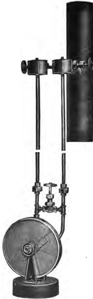
FIG. 81.—Indicating flow meter, type I, form F for measuring steam flow.
